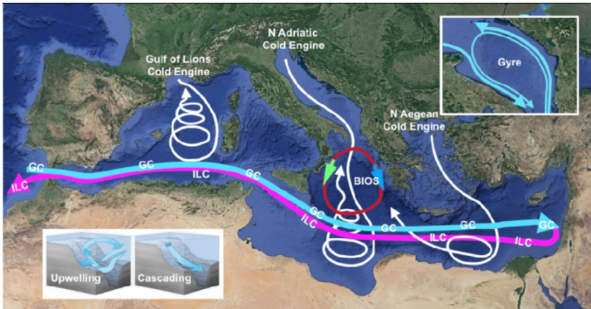
Fig. 6 The main horizontal and vertical currents of the Mediterranean Basin: GC, Gibraltar current; ILC, intermediate Levantine current; BIOS, Bimodal Oscillating System. Lower inset: canyon-generated cascading and upwelling currents. Right inset: gyre generated by coastal morphology. After Danovaro R., Boero F., 2019. Italian seas. In: Sheppard C. (Ed). World Seas. An Environmental Evaluation (second ed.) . Academic Press, London. pp. 283–306.
